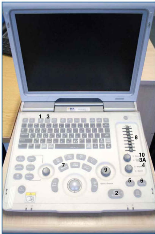
Fig. 16.17. Image of a portable ultrasound machine. Basic keys are indicated: patient details button (1), freeze button (2), exam preset button and probe selection button (3), change the frequency of the probe (3A), depth button (4), save buttons (5, 6), measure button (7), time gain compensation (series of buttons or knobs) (8), overall gain knob (9), focal zone button/ knob (10).
