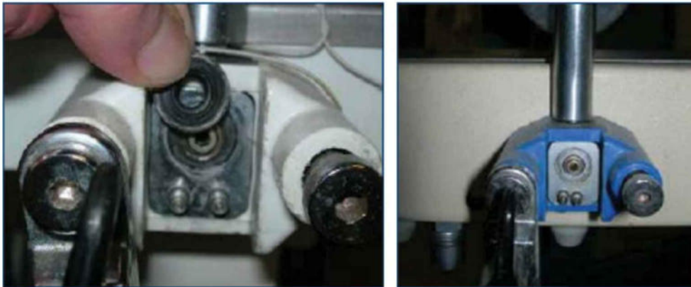
Fig. 7.2. Pin index showing the gas-specific arrangement of pins, which will only fit into the corresponding holes on the correct cylinder.
