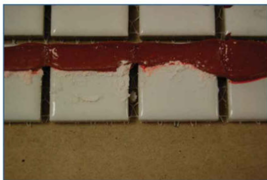
Fig. 23.2. A prototype veterinary dental model constructed using ceramic tiles, silicon sealant and grout to emulate teeth, gingiva and calculus, respectively.
