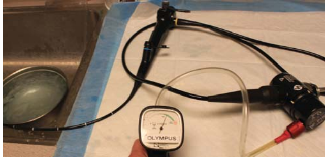
Figure 2.3 Leak testing a videoscope using a hand-held leak tester. The bending section is immersed to look for air bubbles at the A-rubber or from the distal tip, which is a sign of water invasion. Box 2.1 for complete guidelines.
