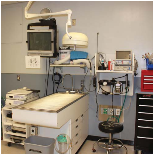
Figure 11.12 One of the endoscopy procedure tables at the VMTH. Ambient light is provided using dimmers on wall lights (above the monitor). Focused task lighting is accomplished with surgical lights on swing arms. A table with a removal grate top is easy to clean. The component tower is mobile to accommodate any endoscopy procedure.
