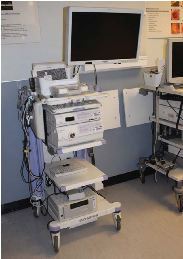
Figure 11.3 A video tower capable of traveling to other parts of the hospital. Set-up includes components for video and all-fiber-optic endoscope and telescope capability, and also adapters for different manufacturers' endoscopes. An image capture device is also included. The monitor is on a swing arm attached to the cart.
