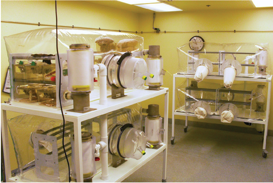
Fig 3.2. Isolator within a gnotobiotic facility containing rodent cages. (Source: Photo courtesy of University of Washington Gnotobiotic Core.)
