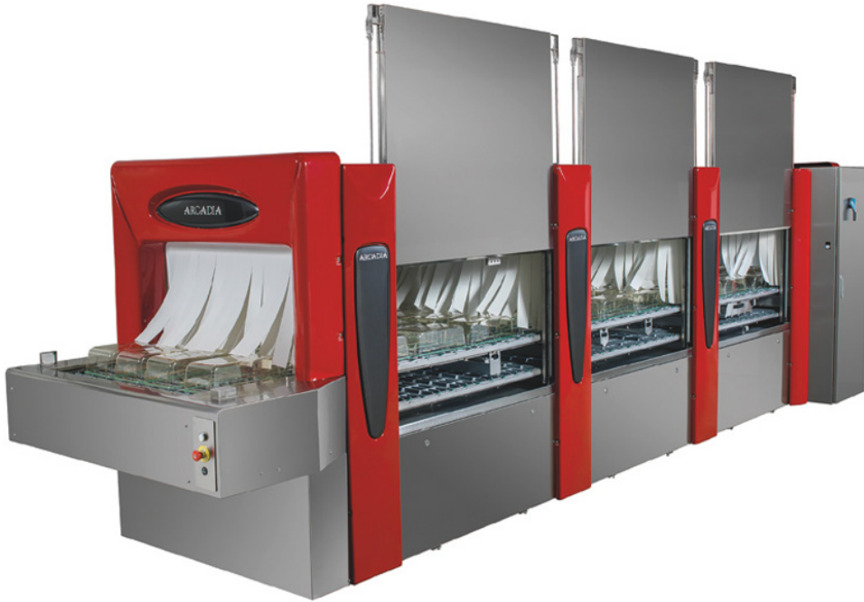
Fig 3.11. Tunnel washer. Side mechanical access panels raised to show three functional areas: the prewash, wash, and rinse sections of the unit through which items are carried on the tunnel's conveyor belt. (Source: Photo courtesy of Tecniplast.)
