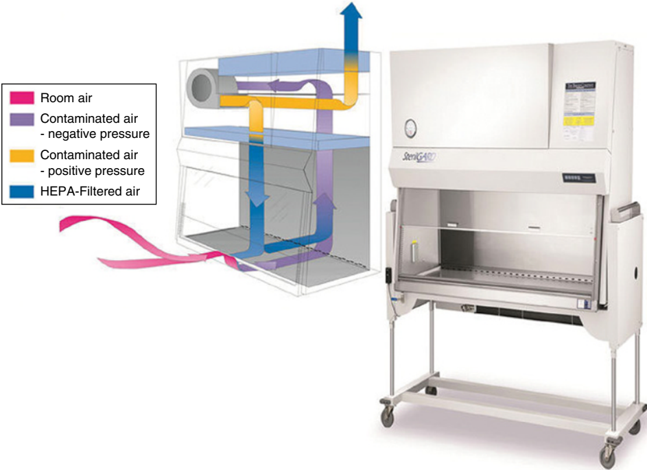
Fig 3.16. Class II – Type A2 Biological Safety Cabinet. Biological safety cabinets (BSCs) provide HEPA filtration of air exhausted from the unit. Class I, II, and III BSCs differ in their containment capabilities and performance features. Class II BSCs are most frequently utilized in laboratory animal facilities. (Source: Images courtesy of The Baker Company, www.bakerco.com .)
