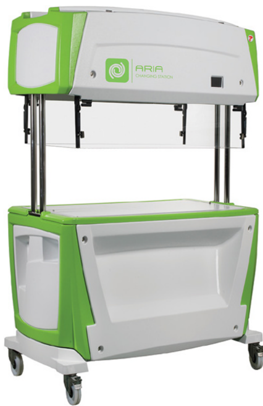
Fig 3.15. Mobile laminar flow hood. In this unit, used for handling rodent caging, HEPA filtered air is directed from the top of the unit, downward toward the work surface. (Source: Photo courtesy of Tecniplast.)
